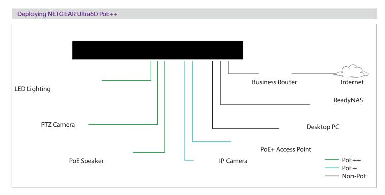
GS516UP and GS524UP can support, but are not limited to, power the devices shown in the above examples.
